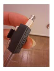
4. Put the replacement fuse into the holder and insert it back into the device
